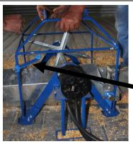
8. Align the **mounting strap** located on the cage leg with the sweep auger back stop and
