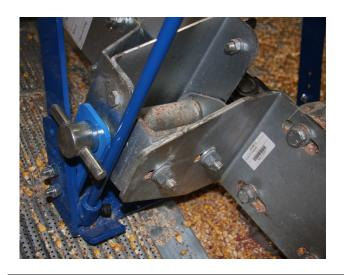
5. Mount the **Sump Saver** back on the **skids** using the bottom holes. Viewing the unit from the outside, the order of parts should be as follows: **skid, Sump Saver leg,** and the **bracket**.
