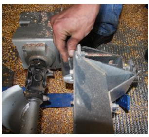
3. Remove the main pin from the sweep and place the **mounting bracket** on the pin.
