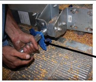
4. Replace the pin. NOTE: The **bracket** will be marked indicating the outside).
